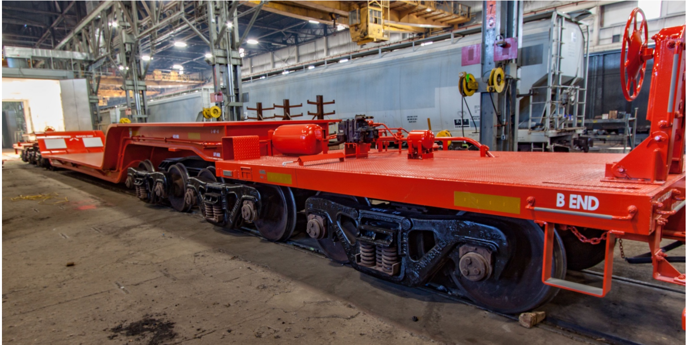
12 Axle Depressed Flat Car subject to net lease is shown RRTX fleet color “International Orange”
